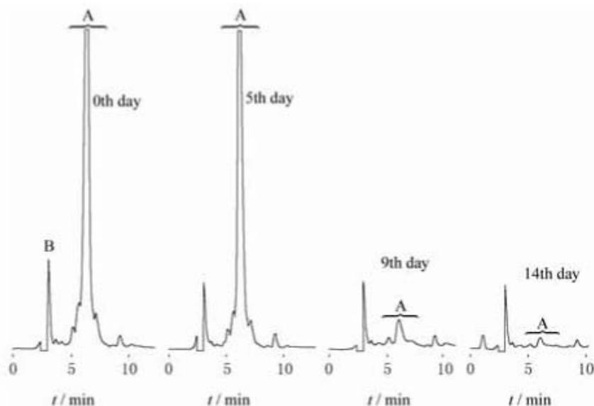
**Fig. 3 HPLC chromatograms of biodegradation intermediates of NP2EO in shaking-flask tests.**
