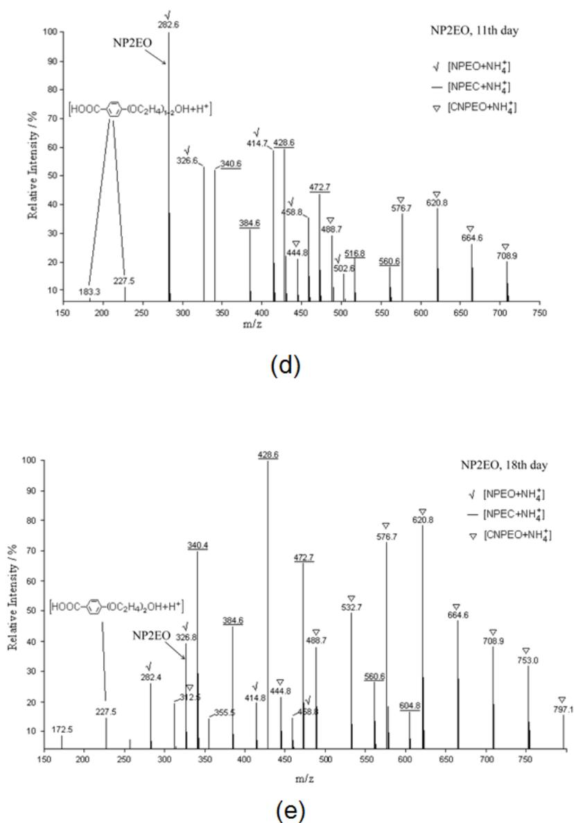
Fig. 5 ESI-MS spectra of NP2EO at degradation time of days 0, 5, 8, 11 and 18.
