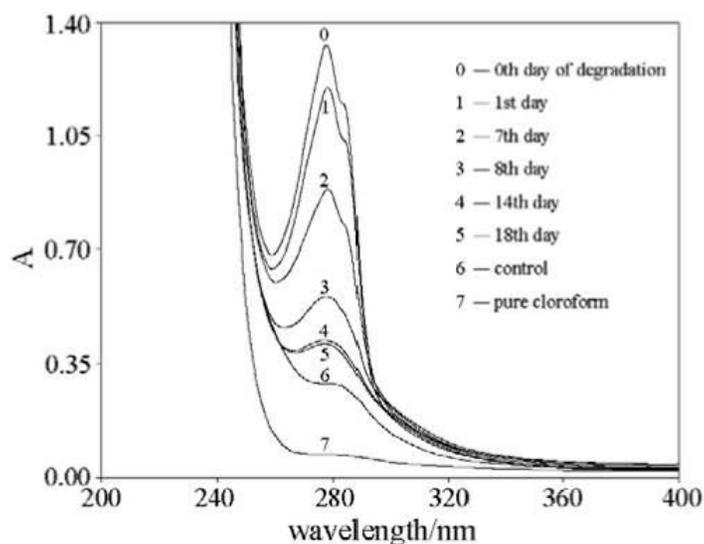
**Fig. 1 UV spectra of chloroform solution of benzene rings of degradation intermediates of NP2EO.** The maximum absorbance is at 277 nm.
