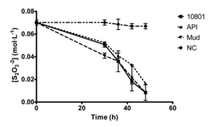
Fig. 2 Thiosulphate consumption (mol L<sup>-1</sup>) vs Time (hrs) of strains isolated in this study and the *T. thioparus* ATCC 10801 strain at 24°C. 10801, ATCC 10801 strain; API, water separator strain; MUD, sludge strain; NC, Negative Control (non inoculated). [ $S_2O_3^{-2}$ ]: Thiosulphate concentration.
