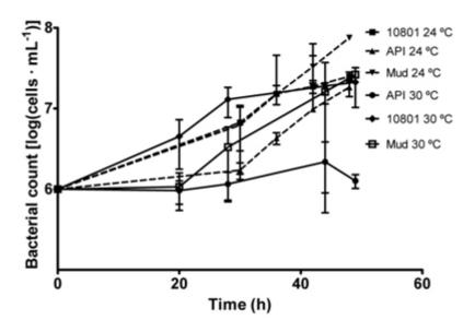
Fig. 1 Growth curves of strains isolated in this study and the *T. thioparus* ATCC 10801 strain at 24°C and 30°C. 10801, ATCC 10801 strain; API, water separator strain; MUD, sludge strain.
