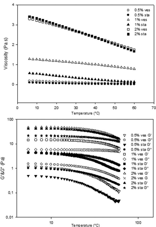
Fig. 3. Viscosity, Storage ( $G'$ ), and Loss ( $G''$ ) modulus change of different gum solutions obtained from *X. axonopodis* pv. *vesicatoria* and *X. campestris* DSM 19000 against temperature.
