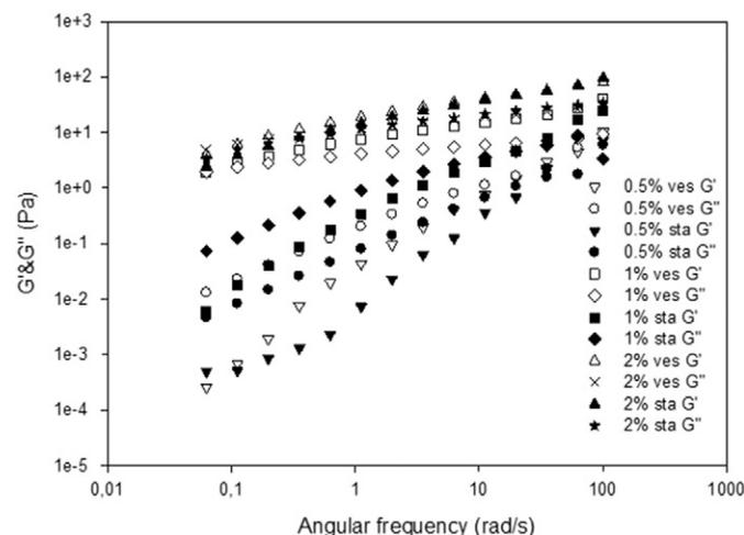
Fig. 4. Storage ( $G'$ ) and Loss ( $G''$ ) modulus change of different gum solutions obtained from *X. axonopodis* pv. *vesicatoria* and *X. campestris* DSM 19000 against angular frequency.
