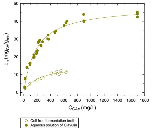
**Fig. 2.** Adsorption isotherms for the adsorption of CA on IRA 400 resin: Aqueous solution of Clavulin® and cell-free fermentation broth, at 25°C and pH 7.0.
