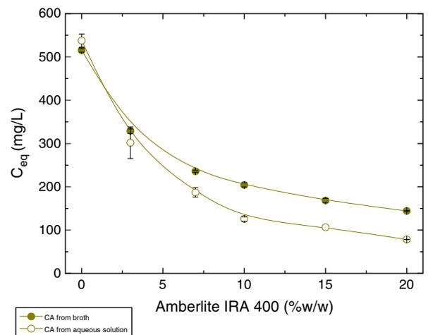
**Fig. 3.** CA concentrations at equilibrium ( $C_{CAe}$ ) as a function of the quantity of IRA 400 used: CA from broth and CA from aqueous solution.
