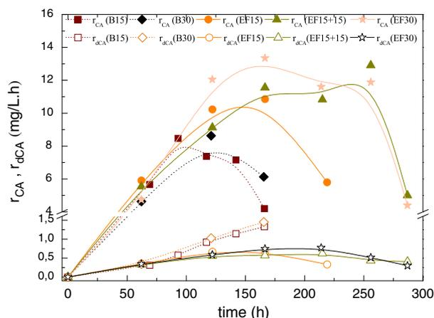
Fig. 7. Profiles of CA production rate ( $r_{CA}$ ) and CA degradation rate ( $r_{dCA}$ ) during conventional (B15 and B30) and extractive (EF15, EF30, and EF15 + 15) fermentations.
