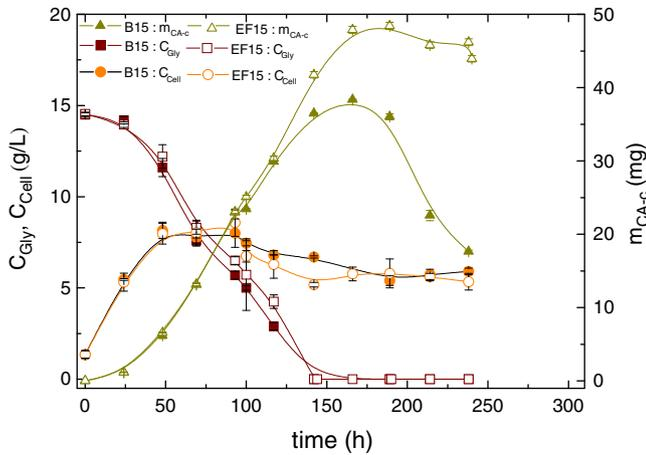
**Fig. 4.** Time courses of glycerol ( $C_{Gly}$ ) and cellular ( $C_{Cell}$ ) concentrations, and cumulative CA mass ( $m_{CA-c}$ ), in the fermentation broth during conventional (B15: control cultivation) and extractive (EF15) fermentations at 20°C with 15 g/L initial glycerol concentration.
