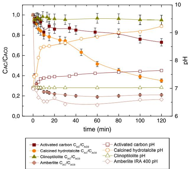
**Fig. 1.** pH profiles and adsorption kinetics using different adsorbents in cell-free fermentation broth containing 500 mg/L of CA.
