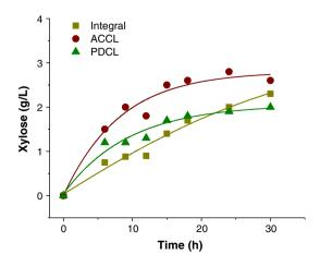
Fig. 2. Xylan enzymatic hydrolysis of different fractions of Arundo donax. ACCL: acid cellulignin; PDCL: partially delignified cellulignin.
