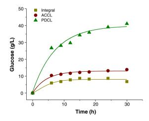
Fig. 1. Cellulose enzymatic hydrolysis of different fractions of *Arundo donax*. ACCL: acid cellulignin; PDCL: partially delignified cellulignin.
