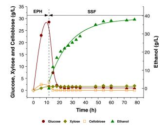
**Fig. 3.** SSF of partially delignified cellulignin of *Arundo donax* with a commercial strain of *S. cerevisiae*. EPH: enzymatic pre-hydrolysis.
